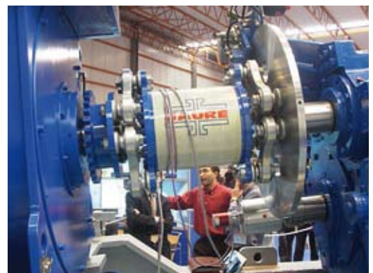
Ixilflex® with JGFS composite spacer.
